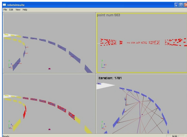
Fig. 5. Test bench used for the plane implementation. The top left shows the mapped planes compared to the actual planes. Top right show the robots perspective of seeing only points, Bottom left shows the results of the EM algorithm to form planes. Bottom right shows the full map with group connectivity
