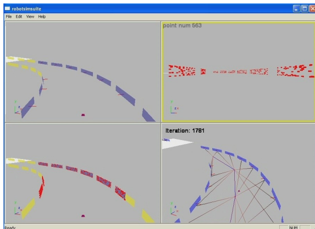
Fig. 6. An example of the simulation used to test the algorithm. The top left window shows the relative map in blue compared to the global map in yellow. The bottom left window shows the output of the EM algorithm compared to the input points. The top right shows the 3D points used as the input. The bottom right shows the connectivity of the relative map
